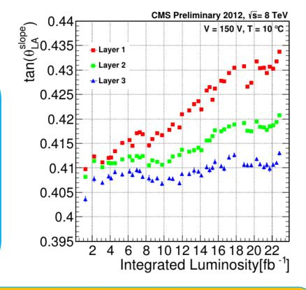
LA also strongly depend on accumulated radiation dose thus we need to measure and upload calibration constants regularly
